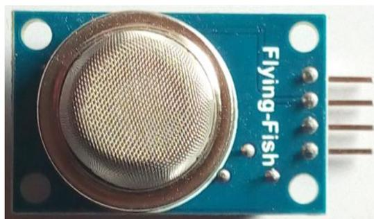
Fig. 3. MQ135 CO<sub>2</sub> Sensor
