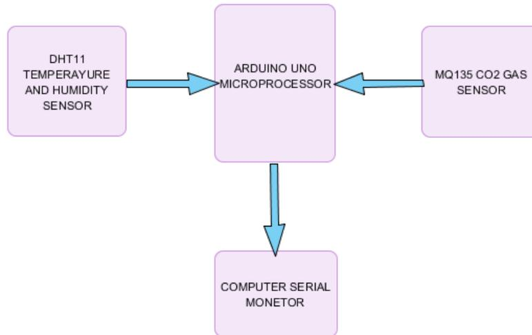
Fig. 6. Block Diagram of the System
